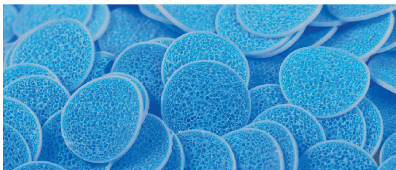
FIGURE 06: Containerized MBBR (top). Biofilm carrier “Mutag Biochips 30TM” used by WTB (bottom). Source: Wastewater Solutions, WTB.
