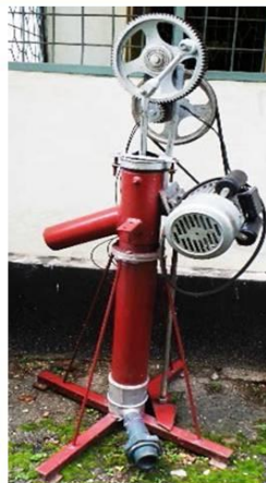
Motorized Gulper Capacity: 90 Liters/min
