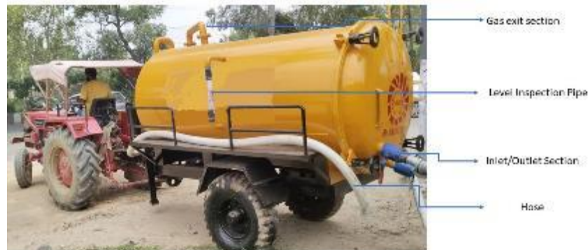
Figure 2-26 A tractor or truck mounted motorized desludging vehicles used in Janakpurdhham Sub-metropolitan City.
