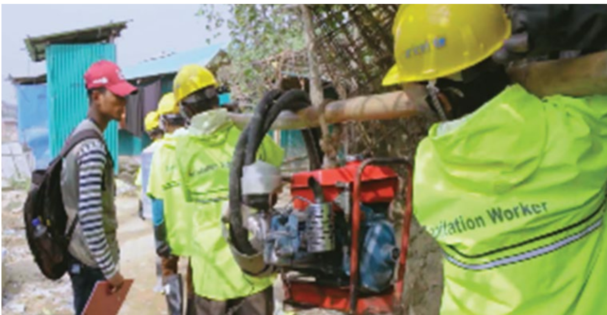
Figure 22: Sanitation workers carrying the hi-cap sucker to the site of operation under the supervision of the volunteer.
